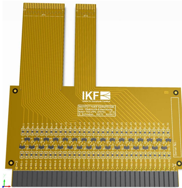
Figure 31: Details of the design of a Kapton adapter cable including the protection circuit.
