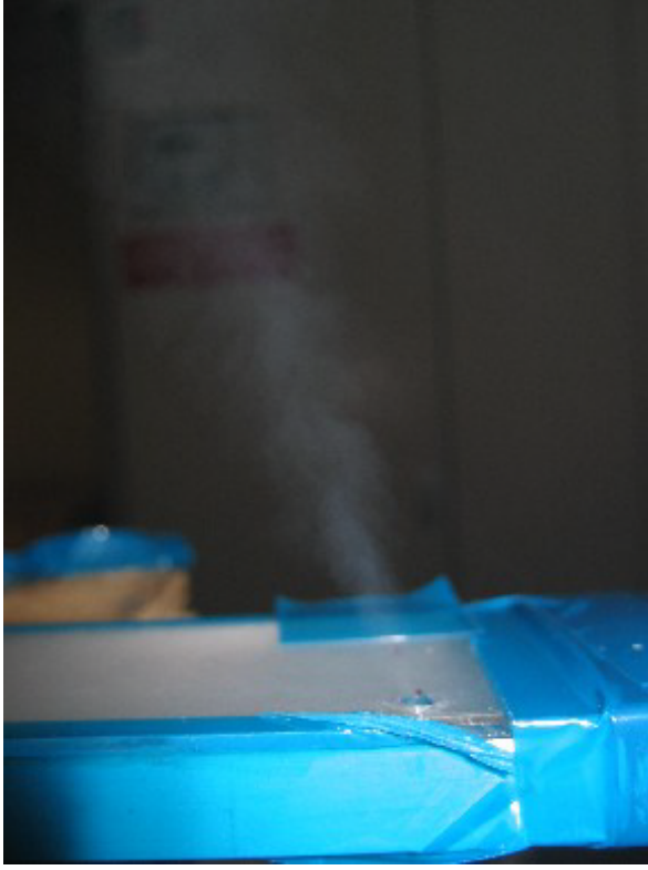
Figure 1: Flow out of the first nozzle of the inlet manifold, for which \frac{Q_{\perp}}{q_{nozzle}} is the highest. The flow out of the upstream half of the hole is null; c_{area} \approx 0.5 .
